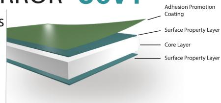
SUPER CLEAR UV STABILIZED THREE LAYER PET FILM, ONE SIDE COATED FOR ADHESION PROMOTION
